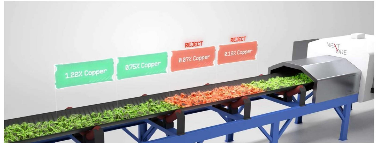
Schematic of NextOre Magnetic Resonance Analyzer
