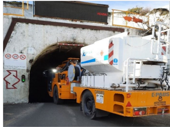
New loading platform developed for Neves-Corvo
