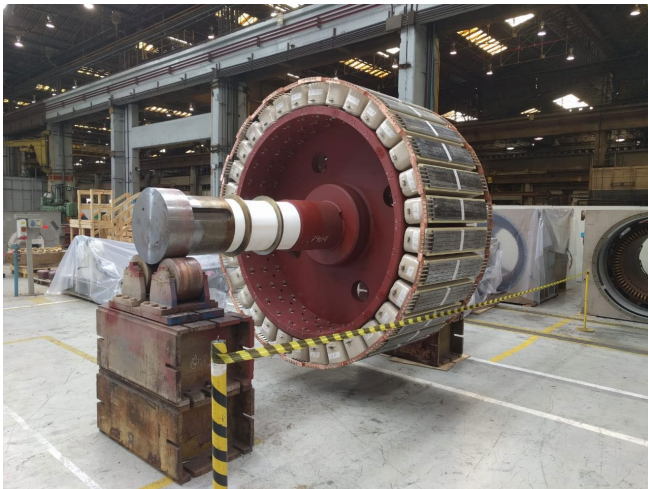
Ball mill motor replacements arriving on site
